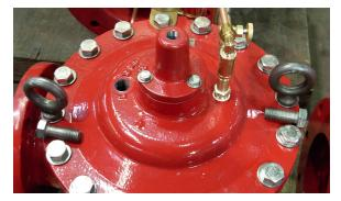
Smaller valves can be lifted by removing two of the cover bolts and replacing with eye bolts temporarily.
