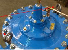
Care should be taken to protect the pilot systems from lifting damage. If necessary this may require spreader bars and slings to eliminate damage to the tubing. If slings are used be careful to position to eliminate the valve spinning in the sling or tipping to cause a safety hazard or causing damage to the pilot system.
